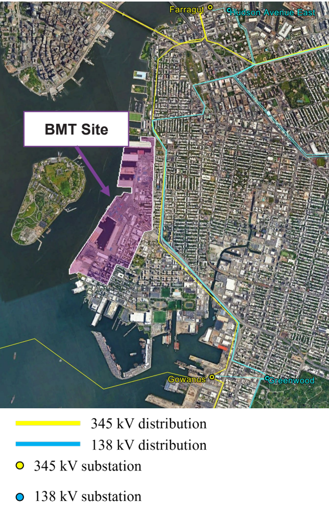
Figure 5: Local Electrical Distribution Near to BMT
